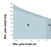
The shape, the height of the gate and the weather conditions can considerably reduce the values shown in the graph to the side.
