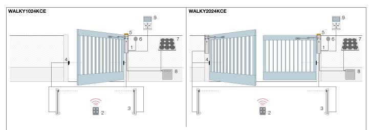
1. Walky 2. Transmitter 3. Photocells mounted on posts 4. Photocells 5. Flashing light 6. Digital or key switches 7. SYP\* solar panel 8. PSY24\* battery box 9. O-View\* multifunction display.
